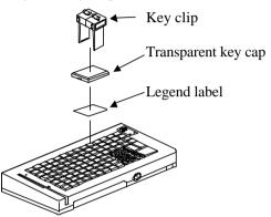
orientate the key tops before they are inserted into the keyboard frame; **failure to do so could result in permanent damage.** Please note that on at least one side of the square stem of the key top, there is a small latching tab to match with a corresponding tab on the bottom inner side of the guide hole as in the example drawing above.
